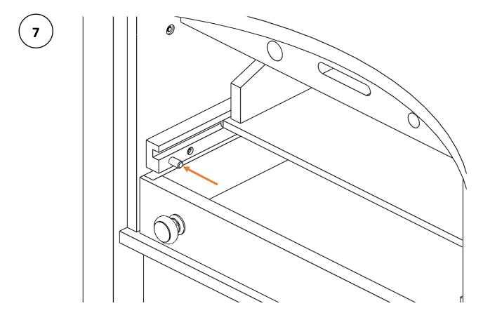
Fit the Tool Holder F to the Bench, as shown below:
