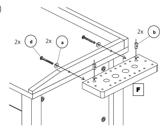
Finally fit the pair of Arm Rests D and Bench Peg E, as shown below:
